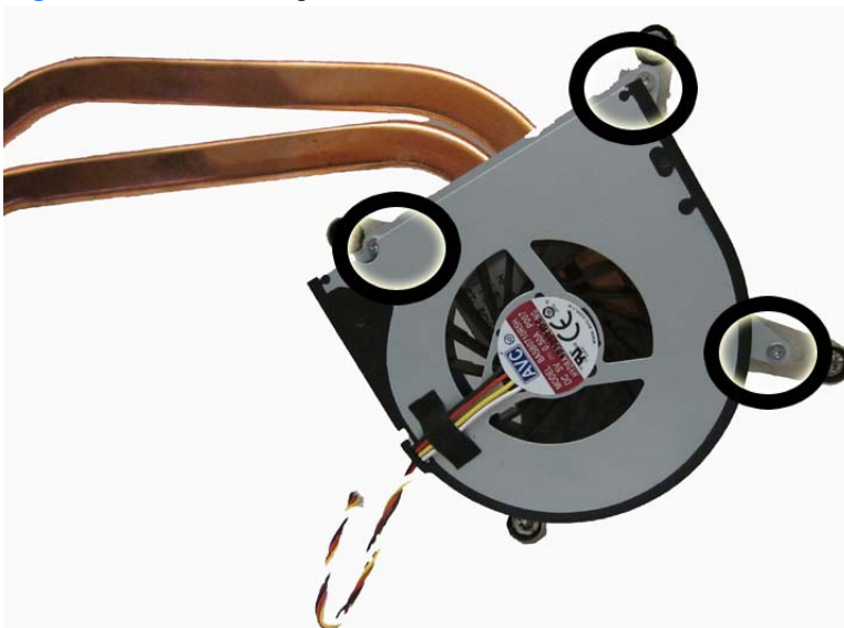
Figure 6-53 Removing the fan from the heat sink
